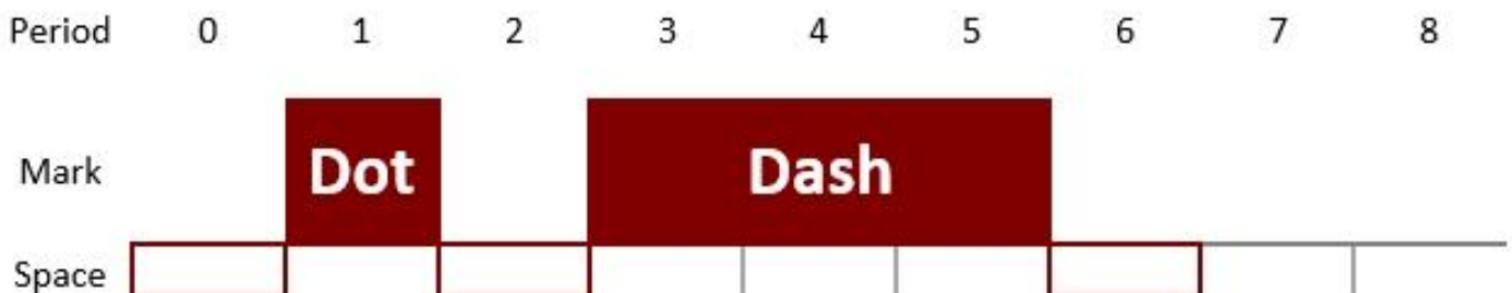
Figure 2 Timing diagram for the letter A in Morse code, based on dot-lengths
